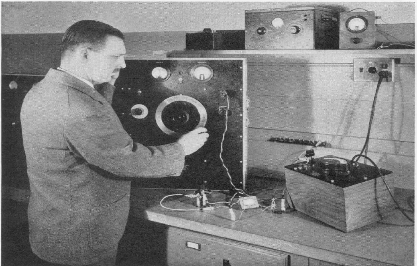
Measuring the response characteristic of an interstage coupling transformer with the TYPE 626-A Vacuum-Tube Voltmeter. The meter is on the bench at the right
